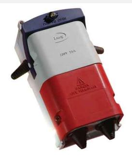
Double pole, single fuse, street lighting cut out for looping up to 6mm <sup>2</sup> 3 core swa cables (when used with a BW gland). Complete with brass cable entry plate with 2 x 20mm holes. Length 150mm, width 81mm, depth 65mm. Rated at 25A maximum. Manufactured & tested to BS7654.
