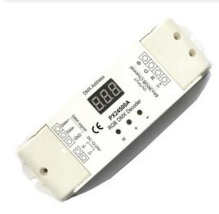
DMX512-RGB 12/24V DC decoder, for converting DMX signals into RGB signals for products such as Flexible LED Strip, LED underwater/landscape lights and LED in-ground lighting. Requires 12 or 24V DC power supply (sold seperately - see LST-PSU). 3 Channel / 6A per channel max hence suitable for 216W @ 12V or 432W @24V
