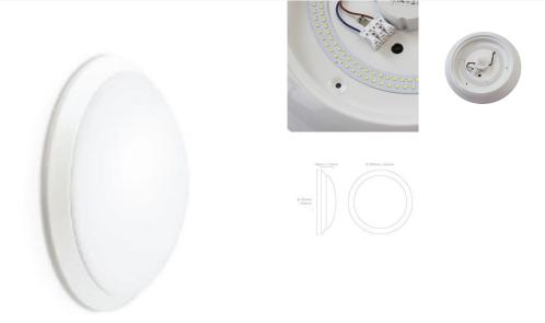
Decorative LED surface mount luminaire designed to replace conventional 2D CFL fittings with 36% energy savings. This fitting comprises of a high quality RAL White power coated aluminium base with a removable PMMA dome diffuser for uniform, stylish light output of up to 2000lm from a series of high quality Epistar SMD 2835 LEDs.
