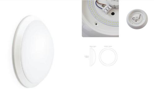
Decorative LED surface mount luminaire designed to replace conventional 2D CFL fittings with 36% energy savings. This fitting comprises of a high quality RAL White power coated aluminium base with a removable PMMA dome diffuser for uniform, stylish light output of up to 2000lm from a series of high quality Epistar SMD 2835 LÉDs.
