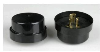
The shorting cap used to replace a NEMA socket photocells when continuity between Li and Lo is required (eg for testing or to make a lantern operate 24/7)
