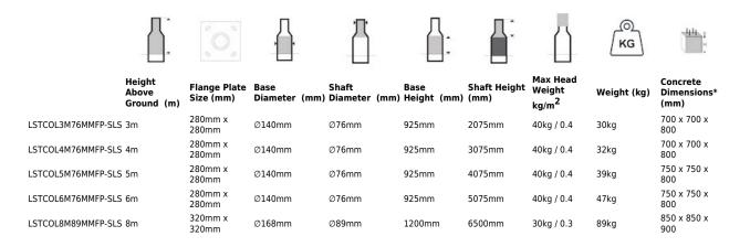
\*Concrete dimensions based on a minimum ground bering pressure of 150kN/m<sup>2</sup> per m (Width x Width x Height)
